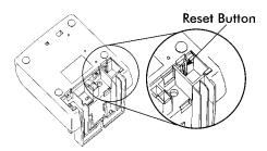
The RESET Button (which is long) is located in the right lower corner on the bottom of the clock.
